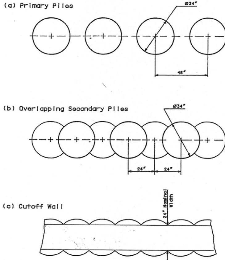
**Figure 10.** Construction sequence for a secant cut-off wall (Bruce and Dugnani, 1995).
