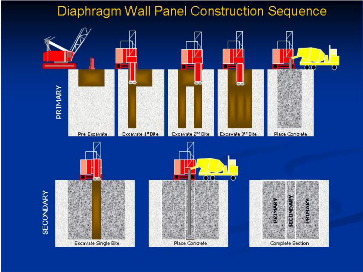
Figure 9. Diaphragm wall panel construction sequence.
