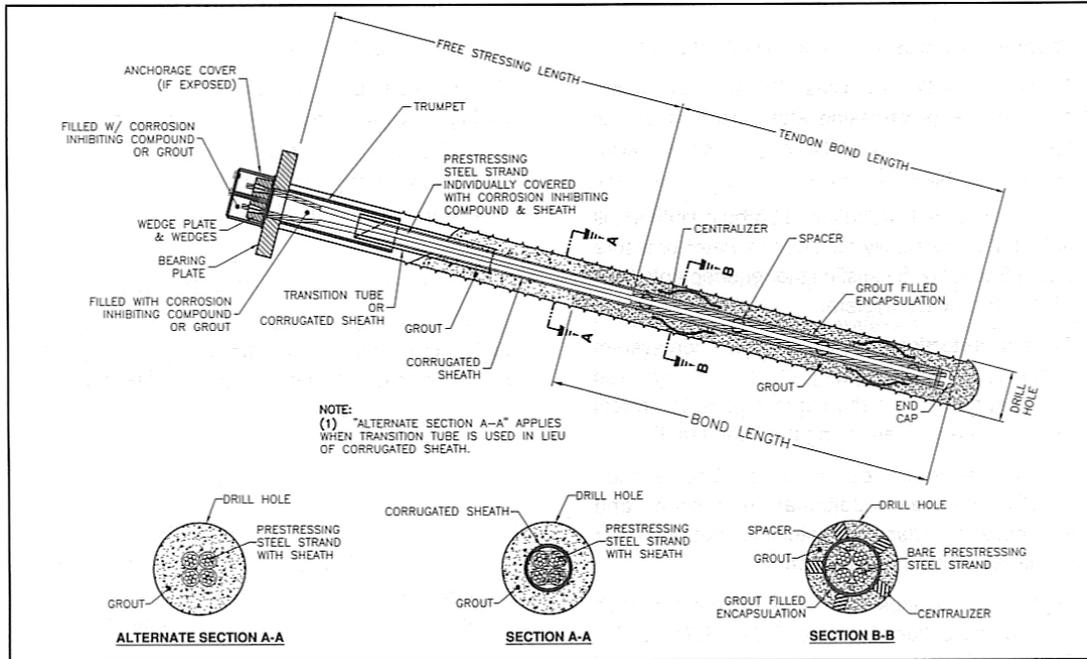
**Figure 2.** Class I Protection – Encapsulated Strand Anchor (PTI, 2004).
