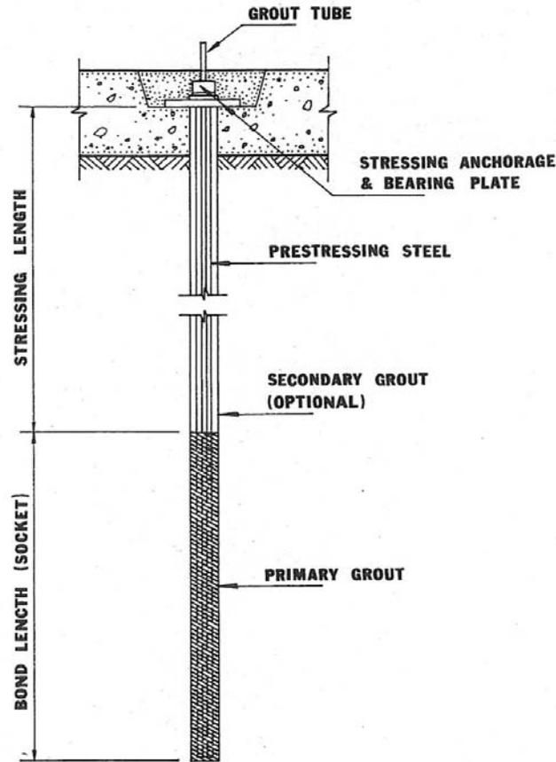
**Figure 1.** Rock Anchor Components (PCI, 1974).
